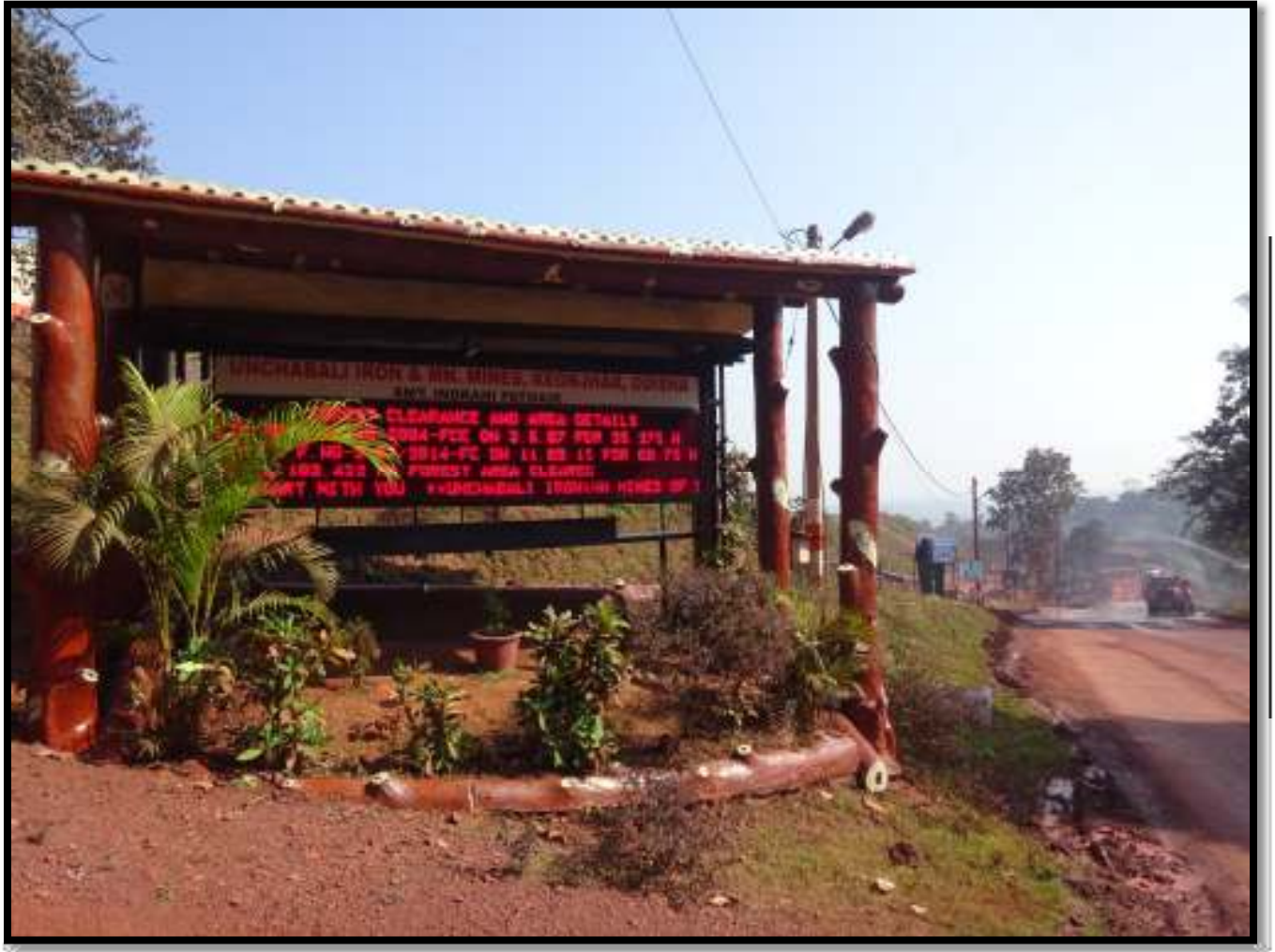
Photo Showing Electronic Display board placed in the mines entrance gate to display the Environmental parameters
