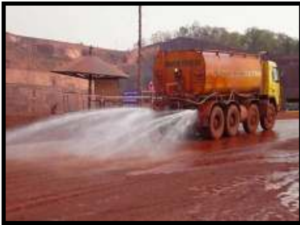
Photos showing mobile water tankers engaged for dust suppression
